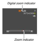
When the zoom pointer reaches the optical/ digital zoom switch over point, it will stop.
